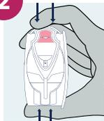
Lock Probe into reaction chamber.
