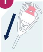
Touch the Smart-Tip Probe™ to the unknown substance, swipe any surface or immerse into the liquid.
