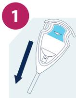
1 Touch the Smart-Tip Probe™ to the unknown substance, swipe any surface or immerse into the liquid.
